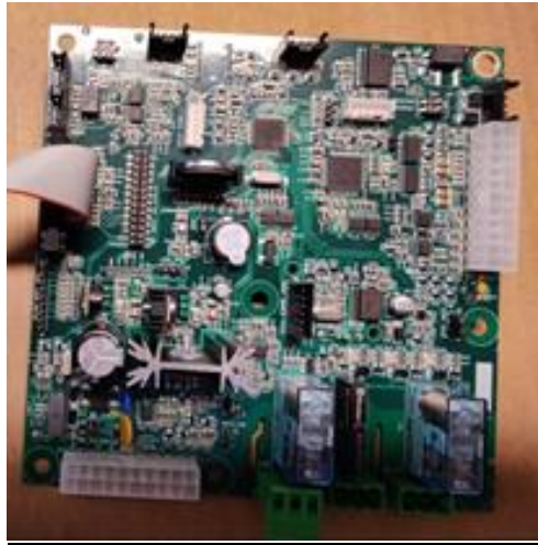
Control Board GE00 (Bottom View)
